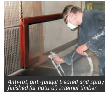
Aluminium to the outside, hardwood timber to the inside
