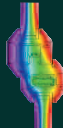
Thermal transfer through Liniar 'A Rated' sash/transom
